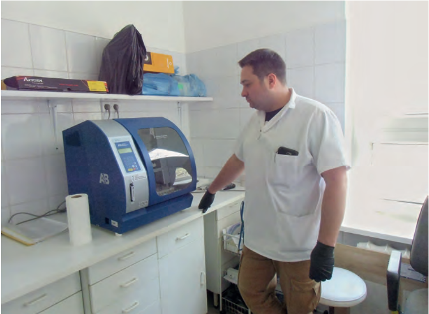
A PCR machine to amplify DNA strands (photo by Karolina Wichowska)
