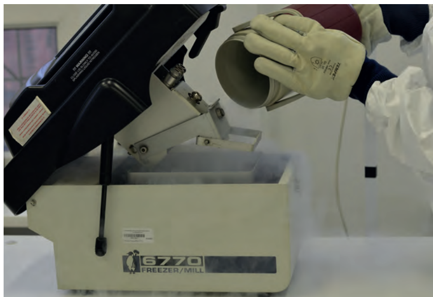
Grinding the bones in liquid nitrogen protects the material from burning (photo by Marta Kuś).
